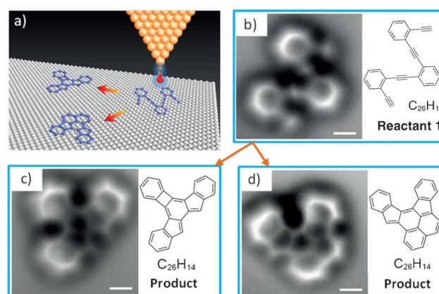
**Figure 1.** a) The tip apex was functionalized with a CO molecule for imaging of the reactant and the final products on the metal surface. b) AFM image of the reactant 1,2-bis[(2-ethynylphenyl)ethynyl]benzene. c, d) Two representative products that were observed after the sample had been heated to 90 °C.<sup>[1d]</sup> Scale bars: 0.3 nm.
