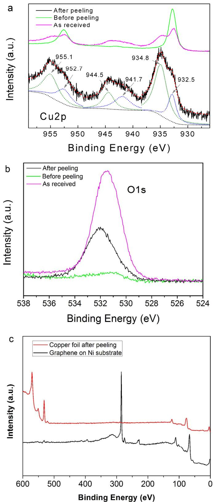
**Figure S1.** XPS measurements of the surface of copper foil. (a) Cu 2p XPS spectra measured on the Cu foil before (solid green line) and after the electrochemical exfoliation (solid black line). The sample
