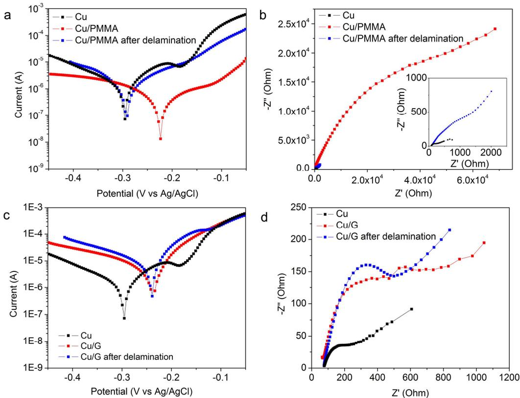
**Figure S2.** The role of PMMA from the control experiments. (a) and (b) Polarization and impedimetric curves of Cu and Cu/PMMA before and after the electrochemical delamination, showing the PMMA layer acts as a corrosion inhibitor. (c) and (d) Polarization and impedimetric curves of Cu and Cu/G, showing no significant change for the Cu/G sample before and after the electrochemical delamination, indicating that the Cu foil is still coated largely by G.
