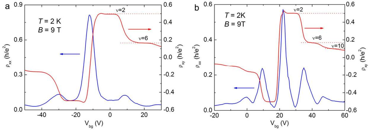
**Figure S4.** Quantum Hall effect for G1 and G2 samples at  $T = 2\text{ K}$  and  $B = 9\text{ T}$ . Graphene samples prepared by three successive electrochemical delamination all shows the fingerprinting quantization sequences of  $\pm(h/4e^2)/(n+1/2)$  for monolayer graphene.
